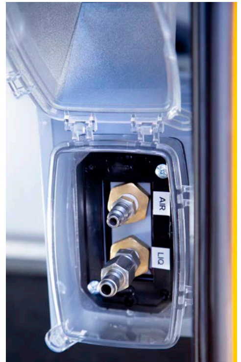
Quick Disconnect Fittings with Protective Enclosure
