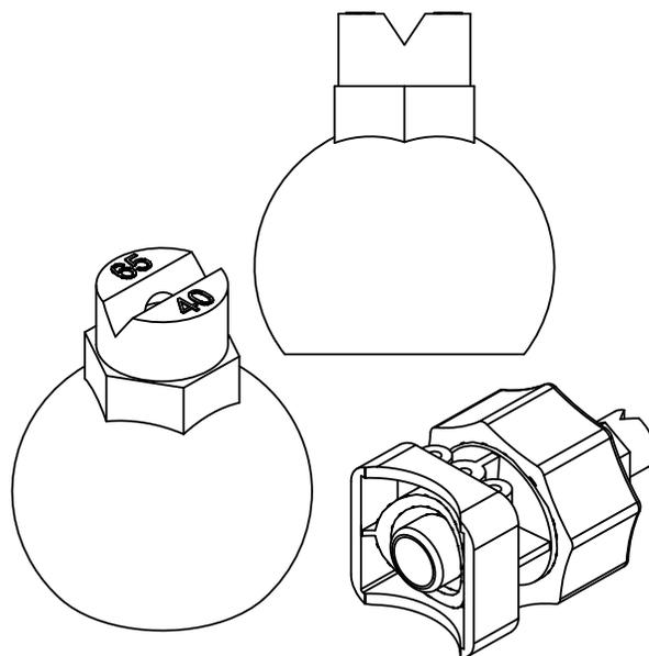
For easy identification, all flat Spray nozzle tips have the tip numbers molded into the ends of the tips.
